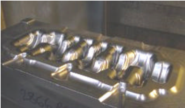
View of the Die after completion of machining
