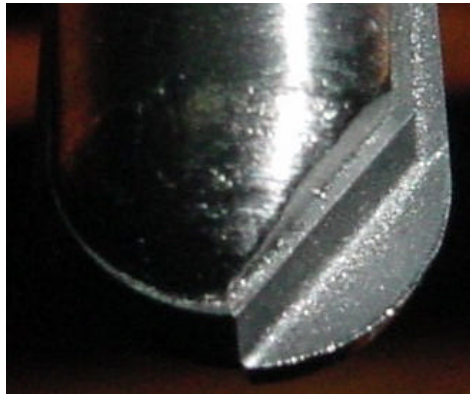
View of Insert wear after completion of machining and tool life
