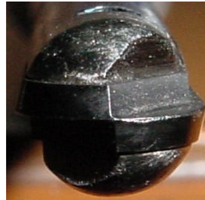
View of Insert wear after completion of machining and tool life
