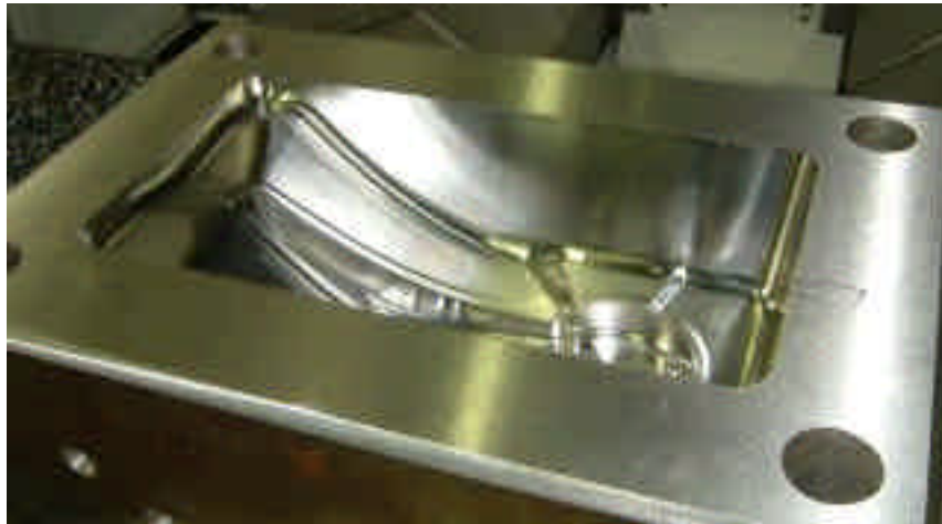
Handle Cavity after completion of Machining
