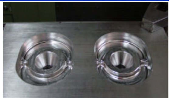
Rubber Mold Cavity after Roughing operation
